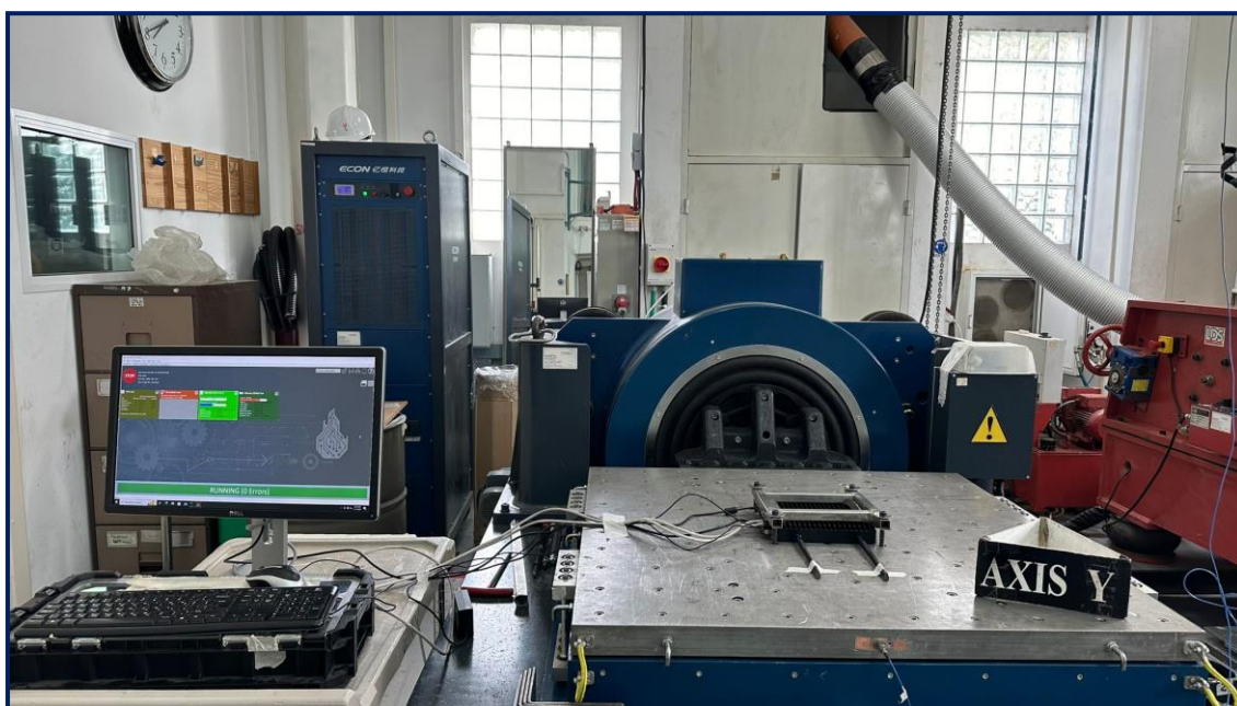
Photograph 6.1.3 Random vibration test setup (longitudinal axis)
