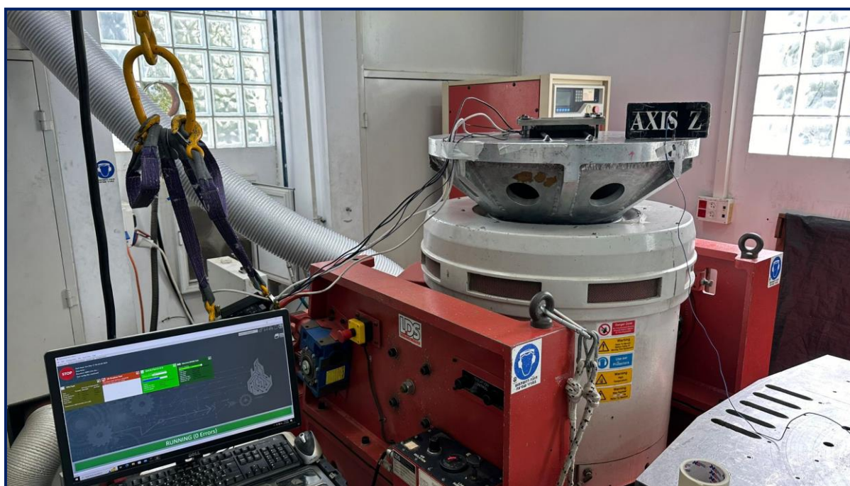
Photograph 6.1.1 Random vibration test setup (vertical axis)
