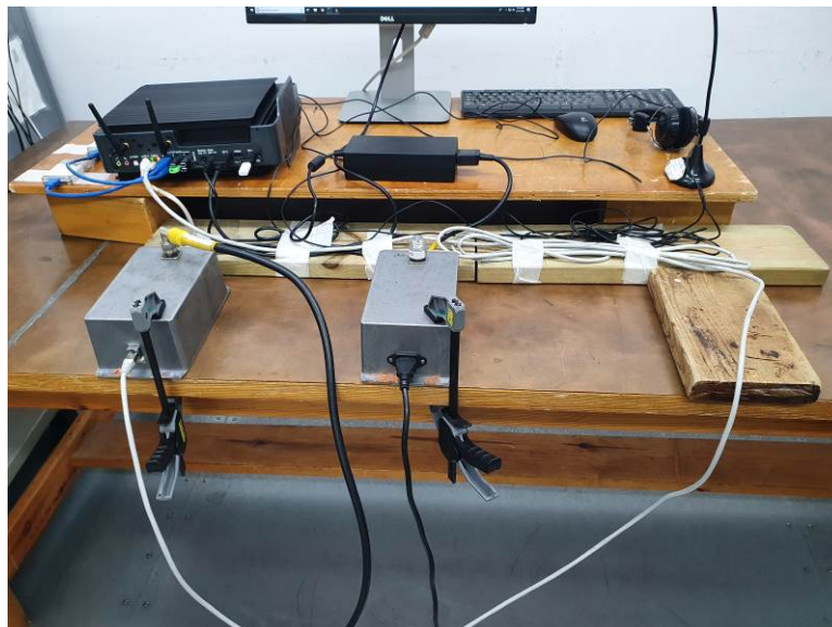
Photograph 9.5.2 Setup for immunity to conducted disturbances induced by radio frequency fields at telecommunication line, CDN injection method
