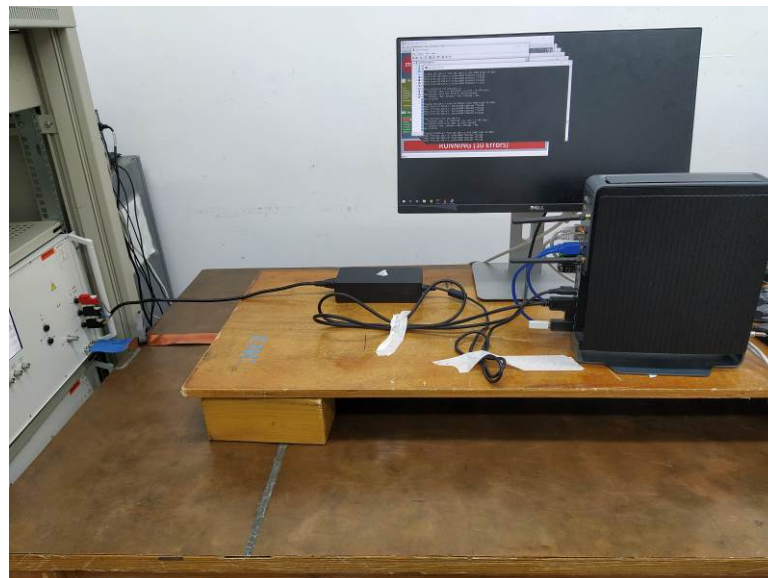
Photograph 9.7.1 Setup for immunity to voltage dips and short interruptions
