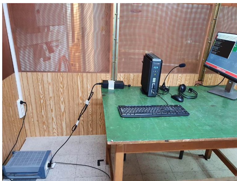
Photograph 8.1.1 Setup for conducted emission measurements at AC mains power port
